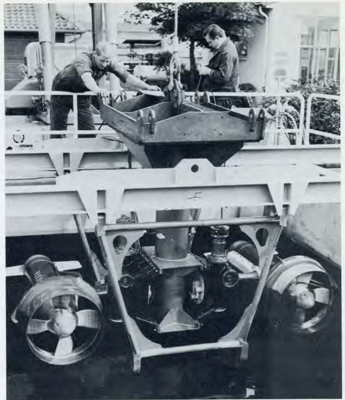
Two of the 25-horsepower AC motors that will be used to propel the PX-15 undergo extensive tests in Hamburg, prior to their shipment to Monthey. Four electrical motors will provide propulsion.
