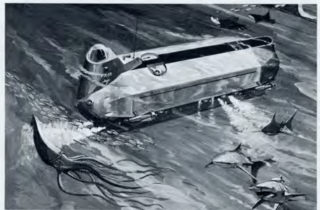
Artist's concept of the PX-15 shows how the new submersible can be used as a stable platform for marine biological, acoustic and other observations at depths to 2,000 feet beneath the surface.
