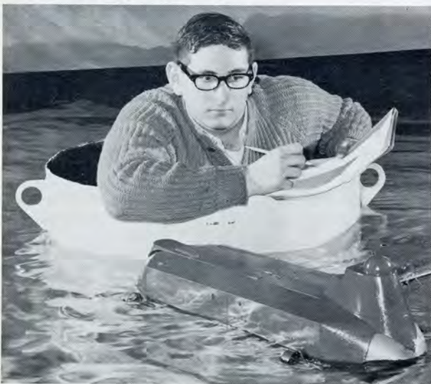
A technician at Stevens Institute of Technology in Hoboken, N.J., checks the hydrodynamic characteristics of a scale model of the Grumman-Piccard PX-15, prior to the start of actual construction.
