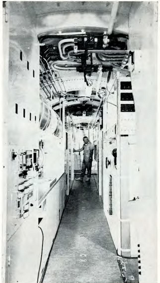
Figure 2. *Franklin* interior—Hull penetrators in overhead and below deck.
