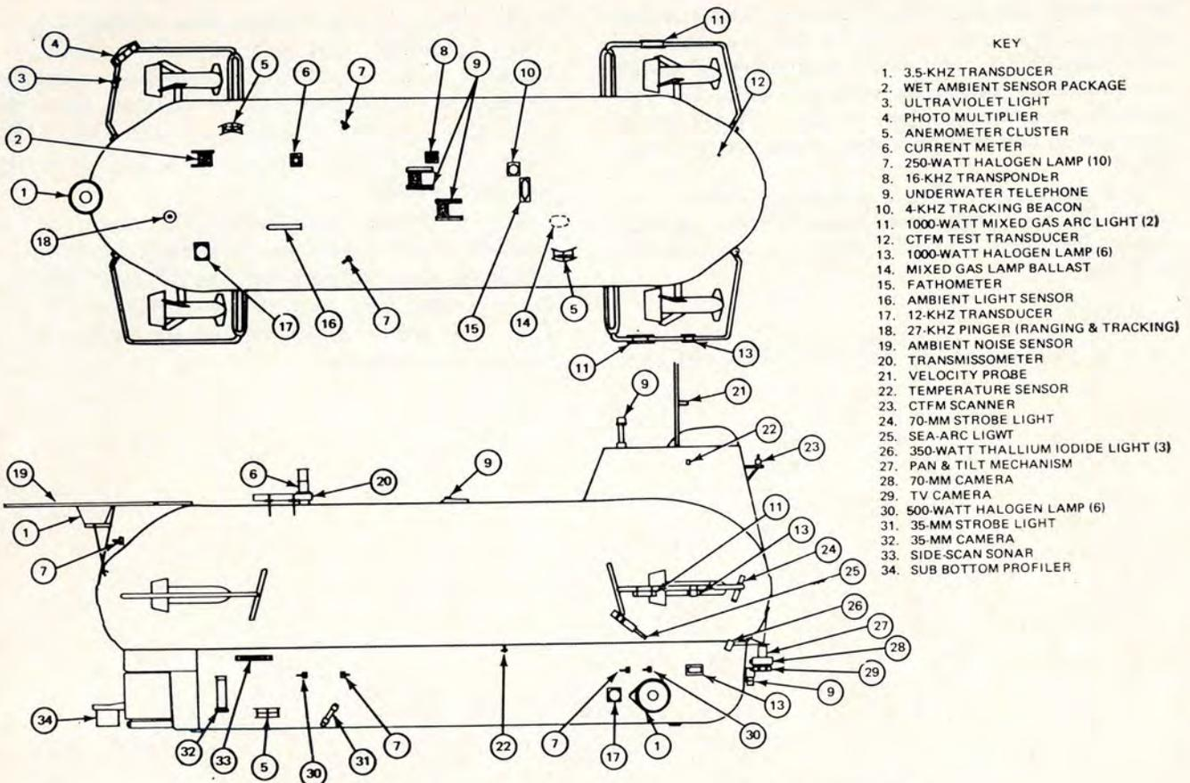
Figure 5. Gulfstream Drift Mission Oceanographic Instrumentation.
