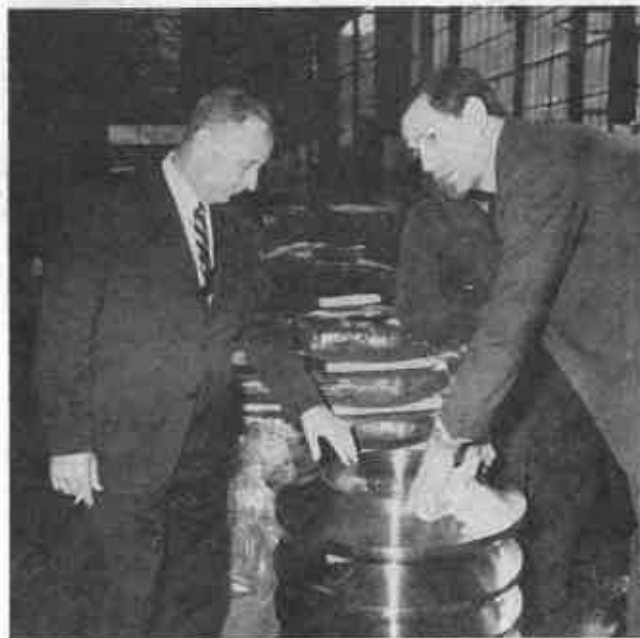
Fig. 6—Capt. Louis DeCamp of the U.S.N. Hydrological Office (left) and Dr. Jacques Piccard examine a prefabricated porthole before its installation. PX-15 will have 30 portholes, including those in hatches.
